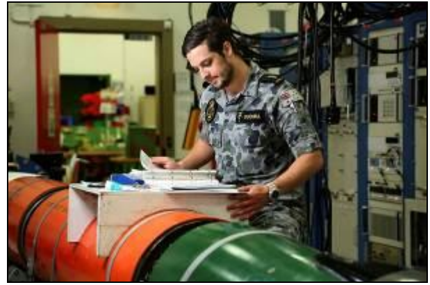
Australian Technician refers to a manual prior to conducting a routine inspection of a Mk 48 Heavyweight torpedo in the Torpedo Maintenance Facility at the Navy Guided Weapons Systems Program Office-West on HMAS Stirling.
