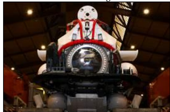
“Nemo”, the Submarine Rescue Vehicle, which forms part of the deployable NATO system.
