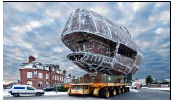
AUDACIOUS forward end construction in transit to Devonshire Dock Hall in 2010
