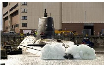
In the water at last - alongside Wet Dock Quay blowing main ballast
